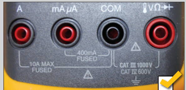
Figure 1. Always verify proper category rating based on location of use. This Fluke 87V is Category III rated for 1000 volts and Category IV rated for 600 volts.
