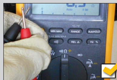
Figure 3. In addition to verifying the DMM operates on voltage, checking continuity of test leads while in the ohms function is always a good idea.
