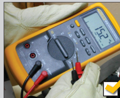
Figure 2. A thorough visual inspection is mandatory. The yellow protective case prevents damage during normal usage.
