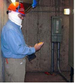
Figure 3. The Fluke iFlex<sup>™</sup> probe has been placed around the incoming 480 V conductor and the disconnect door closed, though not latched. The Fluke 381 clamp meter lies on the floor beneath the disconnect. With the remote display unit removed from the meter, the instructor is able to remain well outside of protective boundaries to observe, demonstrate, and discuss readings.
