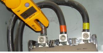
Figure 1. Selecting the proper test equipment for the job is a basic requirement for electrical maintenance, and is identified as such in NFPA 70B. Here we quickly determine that the Fluke TS is too small for the 250 kcmil conductors. On-the-job training, as well as actual maintenance, requires a meter that will provide accurate readings and enhance safety.
