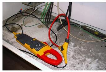
**Figure 2.** One advantage of the iFlex<sup>m</sup> probe is its ability to pass through and around conductors with little disturbance to the conductors. Here the Fluke 381 is lying in the bottom of the AHU VFD cabinet and is connected to read current to the drive. The remote display unit has been removed to allow readings to be taken with the enclosure door closed.
