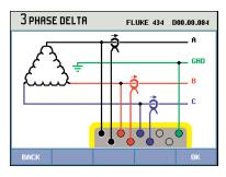
From there, he pushed the Scope button and looked at waveforms and numeric values for all three phases. Judging by the differences between the magnitudes at the top of the screen, there appeared to be a balance problem between the phases.
