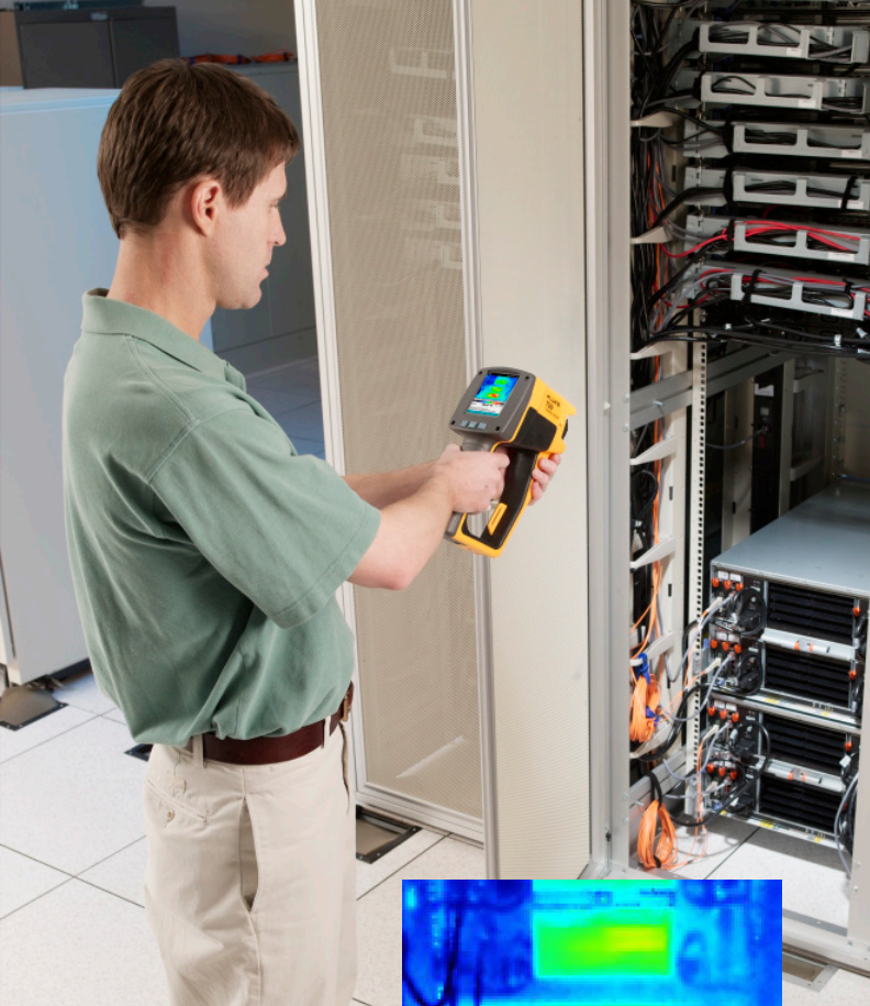
Using the Ti20 to scan heat output from the backside of blade servers.
