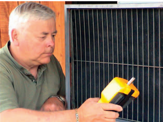
Jim Johnson, a major appliance specialist and instructor, conducts a particle assessment at an air filter.
