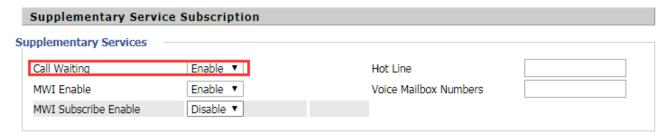
Step 3. At position 1, you can configure whether to enable the call waiting function.
