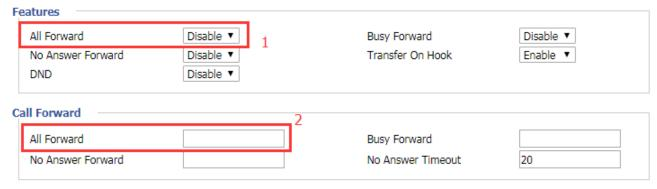
Step 3. Enable all forward at position 1 and fill the destination number at position 2.
