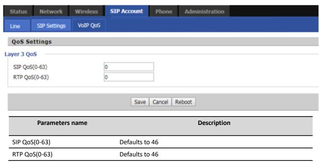
Configuration can be based on the scene environment to modify the parameters
