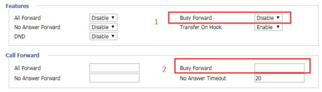
Step 3. Enable the busy forward at position 1 and fill destination number at position 2.
