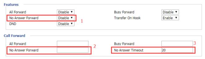
Step 3. Enable the no answer forward at position 1 and fill destination number at position 2.Potion 3 is no answer to the forward time, default 20s.
