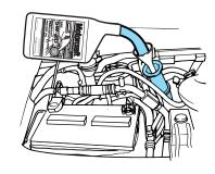
• Do not overfill the engine with oil. Oil levels above this mark may cause engine damage. If the engine is overfilled, some oil must be removed from the engine by an authorized dealer.
