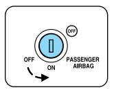
If the OFF light is illuminated when the passenger airbag switch is in the ON position and the ignition switch is in ON, have the passenger airbag switch serviced at an authorized dealer immediately.
