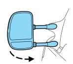
The telescoping feature (if equipped) allows the mirror to extend approximately 3.15 inches (80 mm). This feature is especially useful to the driver when towing a trailer.
