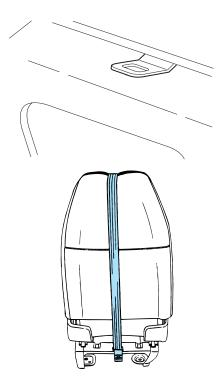
4. Clip the tether strap hook to the seat pedestal to the location shown.
