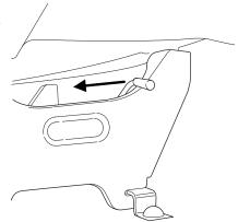
3. Move the seat rearward and lift the seats rear hooks away from the rear strikers prior to lifting the front hooks out from the front strikers.
