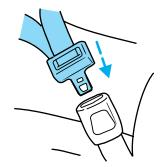
5. To put the retractor in the automatic locking mode, grasp the shoulder portion of the belt and pull downward until all of the belt is extracted.
