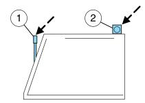
• **Sealed beam:** Locate the vertical adjuster (1) for each headlamp. Adjust the aim by turning the adjuster control either clockwise (to adjust up) or counterclockwise (to adjust down).
