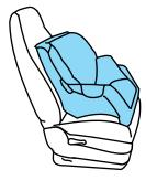
An airbag can kill or injure a child in a child seat. Never place a rear-facing child seat in front of an active airbag. If you must use a forward-facing child seat in the front seat, move the seat all the way back.
