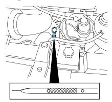
$6. \ \, \text{Wipe}$  the indicator clean. Insert the indicator fully, then remove it again.
