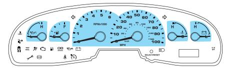
**Speedometer:** Indicates the current vehicle speed.
