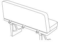
3. Clip the tether strap hook to the tether bracket mounted under rear rail of seat cushion frame.
