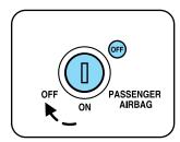
is in the OFF position and the ignition switch is in ON, have the passenger air bag switch serviced at your Ford or Lincoln-Mercury dealer immediately.
