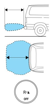
The RSS automatically turns on when the gearshift lever is placed in R (Reverse) and the ignition is ON. An RSS control allows the driver to turn the RSS on and off. To turn the RSS off, the ignition must be ON, and the gear selector in R (Reverse). An indicator light on the control will
