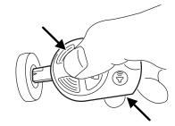
To gain more leverage when rotating the IKT in the ignition lock cylinder, you can readjust the location of your thumb to grasp the IKT on the outer edge next to the control.
