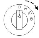
The autolamp system also keeps the lights on for a predetermined
