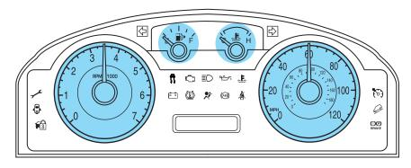
**Speedometer:** Indicates the current vehicle speed.
