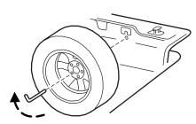
clockwise into the threaded hole in the vehicle until the tire is secured. **If you are stowing the temporary spare tire,** place the tire over the jack and secure it with the large wing nut.
