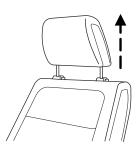
3. Lower the head restraint by pressing and holding the guide sleeve adjust/release button and pushing down on the head restraint.
