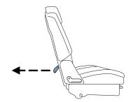
3. To return the seatback to the floor from tumbled position, rotate the seat down until you hear it latching to the floor.
