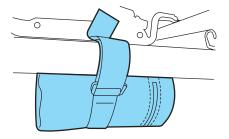
The temporary mobility kit consists of an air compressor to reinflate the tire and a sealing compound in a canister that will effectively seal most punctures caused by nails or similar objects. This kit will provide a temporary seal allowing you to drive your vehicle up to 120 miles (200 km) at a maximum speed of 50 mph (80 km/h).
