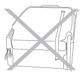
**Note:** In order to allow the seat to latch in the stowed position, do not stow objects under the seat before stowing.
