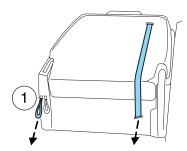
**WARNING:** Ensure seat is latched to vehicle floor by pushing/pulling on seat. If not latched, the seat may cause injury during a sudden stop.
