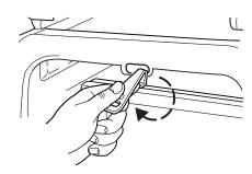
5. Tighten the child safety seat tether strap according to the manufacturer's instructions.
