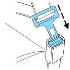
5. To put the retractor in the automatic locking mode, grasp the shoulder portion of the belt and pull downward until all of the belt is pulled out.
