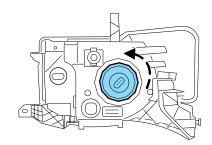
**WARNING:** Handle a halogen headlamp bulb carefully and keep out of children's reach. Grasp the bulb only by its plastic base and do not touch the glass. The oil from your hand could cause the bulb to break the next time the headlamps are operated.
