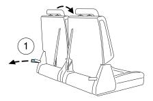
3. From the rear of the vehicle, fold seatback by pulling and holding the number 1 strap while pushing the seatback forward. Release strap once seatback starts rotating forward.
