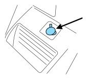
cigar lighter socket is not working, a fuse may have blown. Refer to *Fuses and relays* in the *Roadside Emergencies* chapter for information on checking and replacing fuses.
