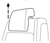
2. Press and hold the unlock/remove button, then pull up on the head restraint.
