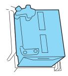
If your battery has a cover/shield, make sure it is reinstalled after the battery has been cleaned or replaced.
