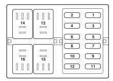
The relay box is located in the engine compartment next to the power distribution box.
