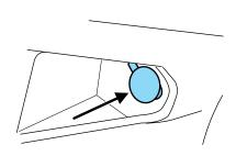
A third rear auxiliary power point is located on the rear of the center console which is accessible from the second row seat.
