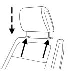
Properly adjust the head restraint so that the top of the head restraint is even with the top of your head and positioned as close as possible to the back of your head. For occupants of extremely tall stature, adjust the head restraint to its full up position.
