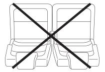
**WARNING:** Do not drive the vehicle when the third row seat is rotated backwards. During a sudden stop, the safety belts are not functional in this position, and during a sudden stop, the third row seat can rapidly tip back to the forward position, all of which may result in serious injury.
