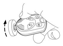
Likewise, when rotating the IKT to the off position in the ignition lock cylinder, the bottom edge of the IKT adjacent to the acountrol can be utilized.
