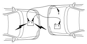
4. Make the final connection of the negative (-) cable to an exposed metal part of the stalled vehicle's engine, away from the battery and the carburetor/fuel injection system. **Do not** use fuel lines, engine rocker covers or the intake manifold as *grounding* points.
