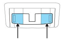
Your vehicle may have reading lamps within the rear dome lamp(s). Press the switches on either side of the dome lamp to turn on the lamps.
