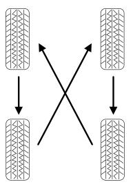
• Rear Wheel Drive (RWD) vehicles/Four Wheel Drive (4WD)/All Wheel Drive (AWD) vehicles (front tires at top of diagram)
