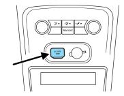
The 110 VAC power point is located on the back of the center console.
