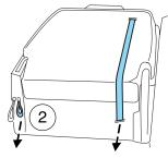
4. Release the cushion latches by pulling the number 2 strap while pulling on the strap located at the top of the seatback to tumble the seat all the way into the tub in the floor.
