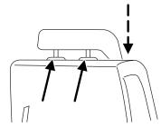
Properly adjust the head restraint so that it is located directly or as close as possible behind your head.
