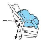
be no more than one inch (2.5 cm) of movement for proper installation.
