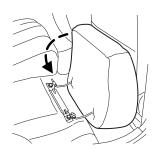
**WARNING:** Before returning the seatback to its original position, make sure that cargo or any objects are not trapped behind the seatback. After returning the seatback to its original position, reinstall the head restraints, and pull on the seatback to ensure that it has fully latched. An unlatched seat may become dangerous in the event of a sudden stop or collision.
