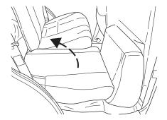
2. Rotate seat cushion down into the seating position making sure that the seat cushion is locked into place and that the safety belt buckles are exposed.
