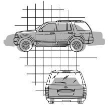
quicker to respond to steering inputs than a vehicle with a longer wheelbase.
