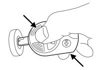
To gain more leverage when rotating the IKT in the ignition lock cylinder, you can readjust the location of your thumb to grasp the IKT on the outer edge next to the control.
