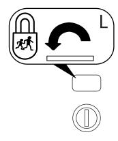
Insert the key and turn in the direction of arrow shown on the door to engage the child proof lock. Turn in the opposite direction to disengage childproof locks.
