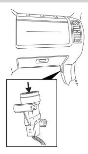
The high voltage shut-off switch is located in the cargo area on the passenger side of the vehicle in the jack compartment, behind the jack access door. The switch is located behind the jack.
