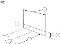
3. Turn on the low beam headlamps to illuminate the wall or screen and open the hood. Cover the left-hand headlamp with an opaque cloth.
