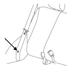
5. To release seatback, pull the seatback release lever (on top of seat) toward the front seat. This is common for both 60% and 40% seatbacks.
