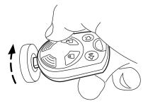
Likewise, when rotating the IKT to the off position in the ignition lock cylinder, the bottom edge of the IKT adjacent to the accountrol can be utilized.
