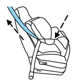
vehicle. Sometimes, a slight lean towards the buckle will additionally help to remove remaining slack from the belt.
