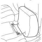
Attach the safety belt web snap button to the quarter trim panel snap button. This will ensure that safety belt does not get caught by staying out of the seat back folding path.
