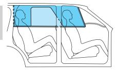
**WARNING:** If the Safety Canopy® system has deployed, the Safety Canopy® will not function again unless replaced. The Safety Canopy® system (including the A, B, C, and D pillar trim and headliner) must be inspected and serviced by an authorized dealer. If the Safety Canopy® is not replaced, it will not function again, which will increase the risk of injury in a future collision.
