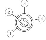
4. Start—starts the engine, vehicle and electrical power systems.
