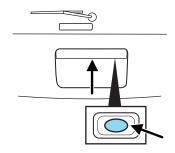
To lock the liftgate and the liftgate window, use the power door locks. Do not open the liftgate or liftgate glass in a garage or other enclosed area with a low ceiling. If the liftgate glass is raised and the liftgate is also opened, both liftgate and glass could be damaged against a low ceiling.
