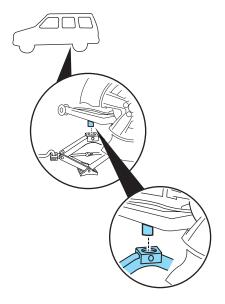
3. Position the jack according to the guides and turn the jack handle clockwise until the tire is a maximum of 1 inch (25 mm) off the ground.
