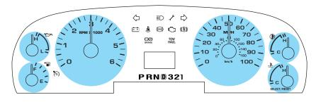
Speedometer: Indicates the current vehicle speed. Vehicle speed is limited to 75 mph (120 km/h).
