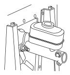
Chassis with Gross Vehicle Weight Ratings of 16,000 lb (7,257 kg) and 18,000 lb (8,165 kg) are equipped with Hydroboost Brake Booster Systems and must use Motorcraft High Performance DOT 3 Motor Vehicle Brake Fluid or equivalent meeting Ford Specification WSS-M6C62-A. Refer to *Maintenance product specifications and capacities* in this chapter.
