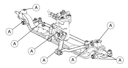
There are nine lubrication points on the steering linkage shown as "A". Refer to *Maintenance product specifications and capacities* in this chapter for lubricant type to use.
