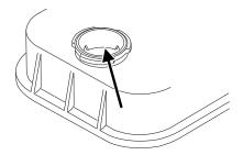
4. Use only a brake fluid listed previously (DOT 3 or Super DOT 4 depending on brake system) and that is certified to meet Ford specifications. Refer to *Maintenance product specifications and capacities* in this chapter.
