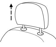
2. Simultaneously press and hold both the adjust/release button and the unlock/remove button, then pull up on the head restraint.
