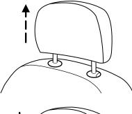
3. Lower the head restraint by pressing and holding the guide sleeve adjust/remove button and pushing down on the head restraint.
