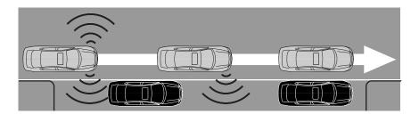
When the system has found a space, the message center will display SPACE FOUND PULL FORWARD followed by a chime. Drive forward until the message center displays SPACE FOUND STOP followed by a chime. When you stop the vehicle in position to begin parking, the message center displays REMOVE HANDS PUT IN REVERSE. The driver should always come to a complete stop before changing gears.
