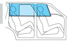
**WARNING:** If the Safety Canopy system has deployed, the Safety Canopy will not function again unless replaced. The Safety Canopy system (including the A, B, C, and D pillar trim and headliner) must be inspected and serviced by an authorized dealer. If the Safety Canopy is not replaced, it will not function again, which will increase the risk of injury in a future collision.
