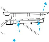
3. Pull the bulb straight out of the socket and push in the new bulb. Install the new bulbs in reverse order.
