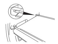
**WARNING:** Ensure that the posts are properly latched in mounting features. The cover may cause injury in a sudden stop or accident if it is not securely installed.
