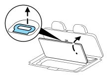
The smaller compartment contains the jack kit. There is also extra storage space for customer use. The lid on the small compartment is accessible and secured by two snap features.
