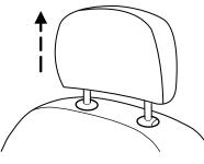
2. Press and hold the adjust/remove button, then pull up on the head restraint.
