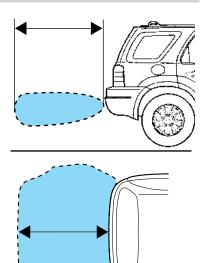
While receiving a warning the radio volume will be reduced to a predetermined level. After the warning goes away, the radio will return to the previous value. The RSS automatically turns on when the gearshift lever is placed in R (Reverse) and the ignition is on. A control in the message center allows the driver to disable the system, refer to Message center in the Instrument Cluster chapter for more information. 228
