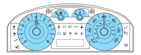
**Speedometer:** Indicates the current vehicle speed.
