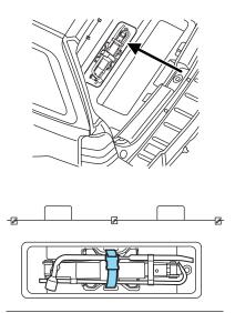
5. Remove the lug wrench from the jack in order to remove the spare tire from under the vehicle.
