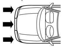
frontal and near-frontal collisions, not rollover, side-impact, or rear-impacts unless the collision causes sufficient longitudinal deceleration.
