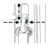
**WARNING:** Position the safety belt height adjusters so that the belt rests across the middle of your shoulder. Failure to adjust the safety belt properly could reduce the effectiveness of the seat belt and increase the risk of injury in a collision.
