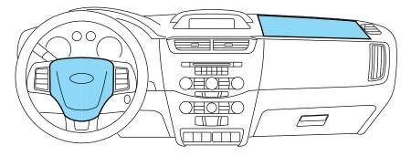
The supplemental restraint system is designed to work with the safety belt to help protect the driver and right front passenger from certain upper body injuries.
