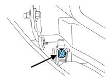
HORIZONTAL AIM IS NOT REQUIRED FOR THIS VEHICLE AND IS NON-ADJUSTABLE.
