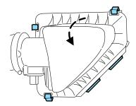
6. Replace the air filter housing cover and secure the clamps. Be sure that the air cleaner cover tabs are engaged into the slots of the air cleaner housing.
