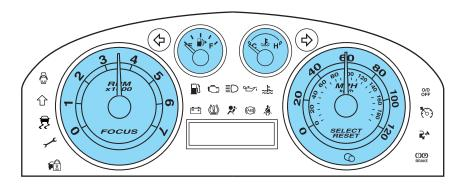
**Speedometer:** Indicates the current vehicle speed.
