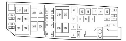
To remove a fuse, use the fuse puller tool provided on the inside of the passenger compartment fuse panel cover.
