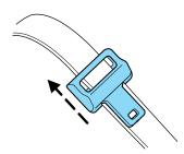
3. While holding both shoulder and lap portions next to the tongue, route the tongue and webbing through the child seat according to the child seat manufacturer's instructions. Be sure that the belt webbing is not twisted.
