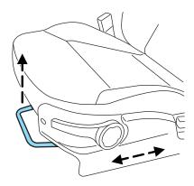
Pull up on the control to raise the seat and push down on the control to lower the seat.
