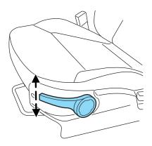
Lift the control to adjust the angle of the seatback.
