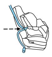
4. Insert the belt tongue into the proper buckle for that seating positions until you hear a snap and feel it latch. Make sure the tongue is securely latched to the buckle by pulling on the tongue.
