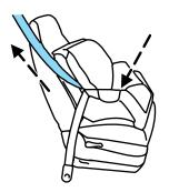
9. Attach the tether strap (if the child seat is equipped). Refer to *Attaching child safety seats with tether straps* later in this chapter.
