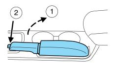
The BRAKE warning lamp will illuminate and will remain illuminated until the parking brake is released.
