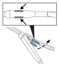
4. Attach the new blade to the arm and snap it into place. Lower the wiper arm and blade back to the windshield. The wiper arms will automatically return to their normal position when the ignition is turned on.
