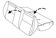
**WARNING:** Before returning the seatback to its original position, make sure that cargo or any objects are not trapped behind the seatback. Make sure that the safety belt is not laying on the seat latch. After returning the seatback to its original position, pull on the seatback to ensure that it has fully latched. An unlatched seat may become dangerous in the event of a sudden stop or collision.
