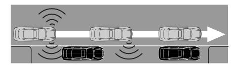
When the system has found a space, the information display will show a corresponding message followed by a chime. Drive forward until the information display shows a corresponding message followed by a chime. When you stop the vehicle in position to begin parking, the information display will show a corresponding message. The driver should always come to a complete stop before changing gears.
