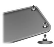
**WARNING:** Always use floor mats that are designed to fit the foot well of your vehicle. Only use floor mats that leave the pedal area unobstructed. Only use floor mats that are firmly secured to retention posts so that they cannot slip out of position and interfere with the pedals or impair safe operation of your vehicle in other ways.
