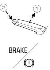
The BRAKE warning lamp will illuminate and will remain illuminated until the parking brake is released.
