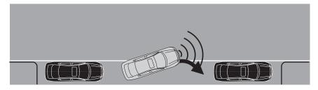
When you determine the vehicle is far enough forward, bring the vehicle to a complete stop and move the gearshift to R (Reverse). Follow the information display instructions. The system may offer subsequent backward and forward maneuvers before proceeding to the finish phase.
