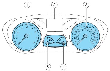
**1. Tachometer:** Indicates the engine speed in revolutions per minute. Driving with your tachometer pointer continuously at the top of the scale may damage the engine.
