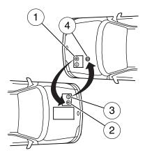
**Note:** Do not attach the negative (-) cable to fuel lines, engine rocker covers, the intake manifold or electrical components as grounding points.
