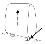
To remove the head restraints, press the unlock/remove button and pull the head restraint up.
