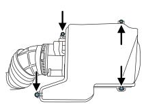
5. Install a new air filter element. Slide the open end of the air filter element in first, below the tab. Then, push the bottom of the closed end in.
