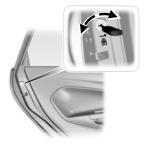
door. Setting the lock for one door will not automatically set the lock for both doors.
