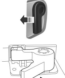
2. Go to the front of the vehicle and locate the auxiliary latch located under the front of the hood (left of center) and then release it by pushing the auxiliary latch to the right.
