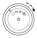
**Note:** If the vehicle is equipped with autolamps, it will have the *windshield wiper rainlamp feature*. When the windshield wipers are turned to low- or high-speed wiping during daylight, and the headlamp control is in the autolamp position, the exterior lamps will turn on after a brief delay and will remain on until the wipers are turned off.
