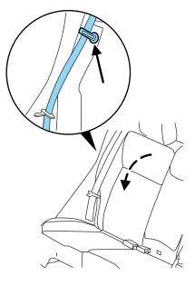
When raising the seatback(s), make sure you hear the seat latch into place and that no red portion is visible on the release button on both sides.
