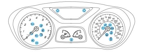
Warning lights and gauges can alert you to a vehicle condition that may become serious enough to cause expensive repairs. A warning light may illuminate when a problem exists with one of your vehicle's functions. Many lights will illuminate when you start your vehicle to make sure they work. If any light remains on after starting the vehicle, refer to the respective system warning light for additional information.
