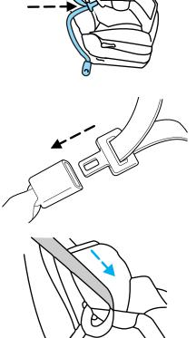
5. To put the retractor in the automatic locking mode, grasp the shoulder portion of the belt and pull downward until all of the belt is pulled out.
