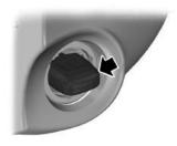
key into the backup location on the steering column. After inserting the IA key into the backup location, use the START/STOP button and brake pedal (automatic transmission) or clutch pedal (manual transmission) to start your vehicle as usual. The vehicle should respond normally as long as the IA key is at the backup location on the steering column. Once the vehicle is started, the IA key can be moved from the backup location, if desired.
