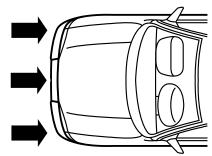
means the forces were not of the type sufficient to cause activation. Front airbags are designed to activate in frontal and near-frontal collisions, not rollover, side-impact, or rear-impacts unless the collision causes sufficient longitudinal deceleration.
