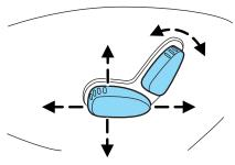
• Push the top of the vertical control forward or rearward to move the seatback forward or backwards.
