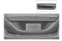
1. Unlock the trunk with the remote control or power door lock control. The trunk will unlock when you press the release button if the intelligent access transmitter is within 3 feet (1 meter) of the trunk.
