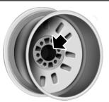
**Note:** Inspect the wheel pilot bore and mounting surface prior to installation. Remove any visible corrosion or loose particles.
