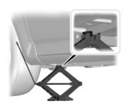
7. Position the jack in the indentions on the sill next to the tire you are changing. Turn the jack handle clockwise until the tire is off the ground.
