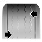
When the tread is worn down to 1/16th of an inch (2 millimeters), tires must be replaced to help prevent your vehicle from skidding and hydroplaning. Built-in treadwear indicators, or wear bars, which look like narrow strips of smooth rubber across the tread will appear on the tire when the tread is worn down to 1/16th of an inch (2 millimeters).
