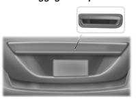
Press the exterior release button above the license plate.
