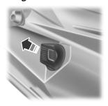
1. Turn the bulb holder counterclockwise and remove it.
