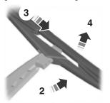
1. Lift and hold the wiper blade off the glass.
