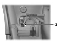
2. Turn the bulb holder counterclockwise and remove it.
