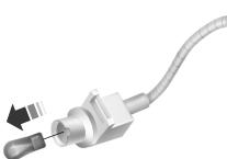
2. Remove the bulb from the bulb holder.
