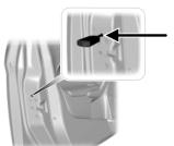
If the central locking function fails to operate, the doors can be individually locked using the key in the position shown.
