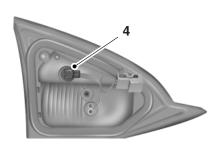
4. Turn the bulb holder counterclockwise and remove it.
