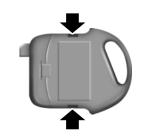
2. Release the retaining clips with a flat object and separate the two halves of the transmitter.
