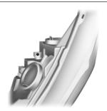
4. Locate the vertical adjuster on each headlamp. Using a Phillips #2 or 13 millimeter wrench/socket screwdriver, turn the adjuster either clockwise or counterclockwise in order to adjust the vertical aim of the headlamp. The horizontal edge of the brighter light should touch the horizontal reference line.
