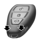
4. Carefully insert a flat object in the position show to open the transmitter.
