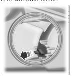
2. Turn the bulb holder counterclockwise and remove it.
