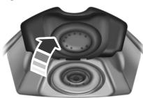
3. Remove the spare tire and jack by turning their tie-down bolts counterclockwise. The lug wrench is located in a bag next to, or on top of, the spare tire.
