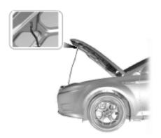
3. Lift the hood and support it with the prop rod.
