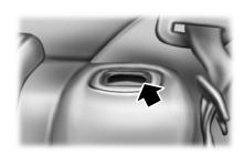
When raising the seat back(s), make sure you hear the seat latch into place and that no red portion is visible on the release button on both sides.
