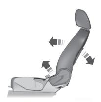
**WARNING:** Reclining the seat back can cause an occupant to slide under the seat's safety belt, resulting in severe personal injuries in the event of a crash.
