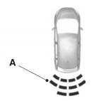
A. Coverage area of up to 6 feet (2 meters) from the rear bumper (with a decreased coverage area at the outer corners of the bumper).
