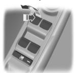
Press the switch to open the window. Lift the switch to close the window.
