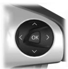
Use the arrows on the right side of steering wheel to navigate through the available menus. Press  $\mathbf{OK}$  to make a selection.
