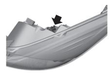
4. Locate the vertical adjuster on each headlamp. Using a Phillips #2 screwdriver, turn the adjuster either clockwise or counterclockwise in order to aim the headlamp. The horizontal edge of the brighter light should touch the horizontal reference line.
