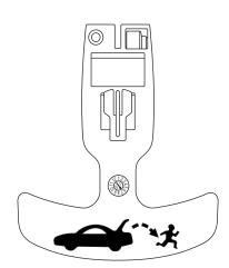
The handle is located inside the luggage compartment either on the luggage compartment door (lid) or near the tail lamps. It is composed of a material that will glow for hours in darkness following brief exposure to ambient light.
