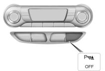
Press the button to switch the system off. It will remain off for the entire ignition cycle.
