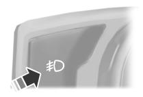
Press the control to switch the fog lamps on or off.
