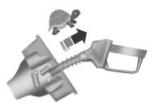
4. After you are done pumping fuel, slowly remove the fuel filler nozzle—allow about five to ten seconds after pumping fuel before removing the fuel filler nozzle. This allows residual fuel to drain back into the fuel tank and not spill onto the vehicle.
