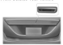
Press the release button located above the license plate. Your vehicle must be unlocked or the intelligent access transmitter must be within 3 feet (1 meter) of the trunk.
