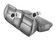
For additional cargo space, flip the seat cushions up before folding the seat back. This feature is only available on vehicles with a split folding seat back.
