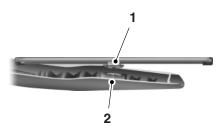
3. To attach the new wiper to the wiper arm, align the slot (1) and cross pin (2) and firmly press the wiper arm into the wiper blade until a click is heard.
