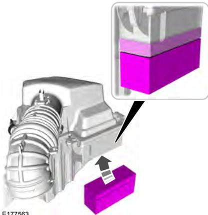
The foam filter must be in place at all times.
