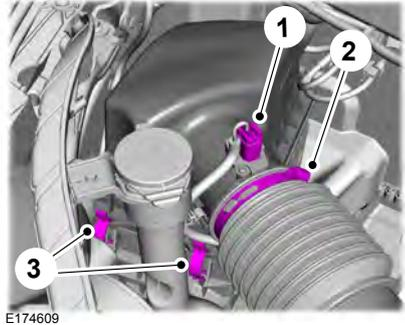
1. Disconnect the mass air flow sensor electrical connector and cable from the air filter cover.
