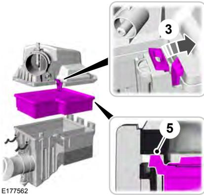
4. Carefully lift the air filter housing cover. Remove the air filter element from the air filter housing.
