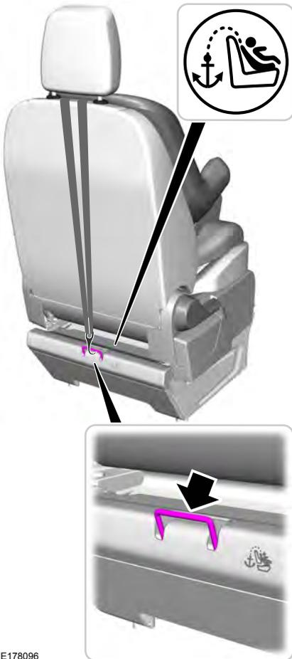
3. Locate the correct anchor on the back panel of the rear seat for the selected seating position. The anchors are labeled with the tether strap symbol and are partially covered by the gap panel. Pull the panel back to fully expose the anchors.
