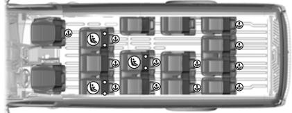
Your vehicle has LATCH lower anchors for child seat installation at the seating positions marked with the child seat symbol.
