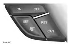
The cruise controls are on the steering wheel.
