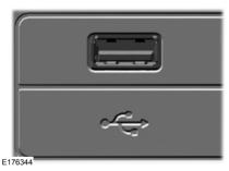
The USB port is located in the center console.
