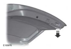
A handle is located inside the liftgate to help with closing.
