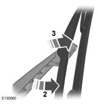
**Note:** Make sure that the wiper arm does not spring back against the glass when the wiper blade is not attached.
