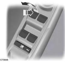
Press the control to open the window.
