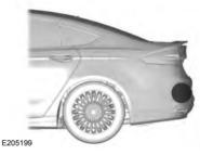
The system uses radar sensors that are located behind the bumper fascia on each side of your vehicle. Any dirt, mud and snow in front of the sensors and/or driving in heavy rain can cause system degradation. Also, other types of obstructions in front of the sensor can cause system degradation. This is referred to as a 'blocked' condition.
