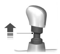
**Note:** The gearshift lever can only be moved to reverse (R) by raising the collar below the gearshift knob up before shifting to reverse. This is a lockout feature which protects the transmission from accidentally engaging reverse (R) when intending to select first (1).
