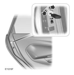
The childproof locks are located on the rear edge of each rear door and must be set separately for each door.
