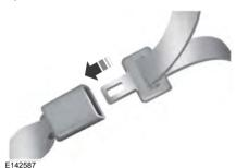
Insert the belt tongue into the proper buckle (the buckle closest to the direction the tongue is coming from) until you hear a snap and feel it latch. Make sure the tongue is securely fastened in the buckle.
