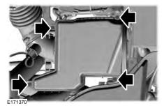
Loosen the four fasteners and remove the air cleaner assembly lid.
