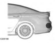
The system uses radar sensors that are located behind the bumper fascia on each side of your vehicle. Do not allow mud, snow or bumper stickers to obstruct these areas, this can cause degraded system performance. See **Blind Spot Information System** (page 166). If the Blind Spot Information System is blocked, Cross Traffic Alert is also blocked. A corresponding message appears in the information display as soon as you shift the transmission into reverse (R).
