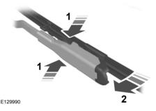
**Note:** Make sure that the wiper arm does not spring back against the glass when the wiper blade is not attached.
