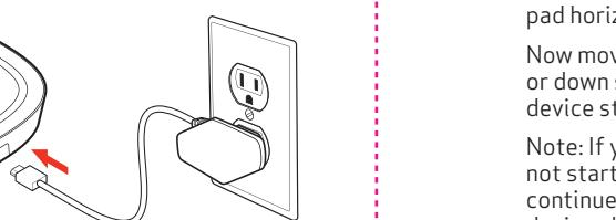
\*Use the included power supply for fastest charging rate. Using a power supply rated under 1.8A will cause the phone to charge slower, indicated by a blinking red LED
