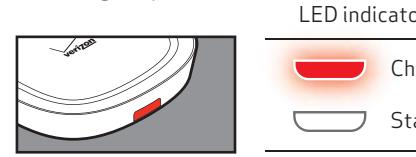
If the red LED is on but no power is being received by the device, there may be a metal object near the coils. Pick up the device and remove foreign objects and place device back on the Verizon Qi Wireless Charging Pad. This is a safety feature and normal operation.
