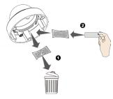
15. Install the dome cover and remove the protective wrap.
