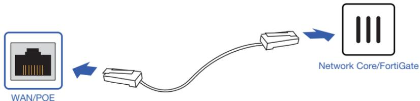
Connect the FortiAP device to a FortiGate controller or an Internet connection.
