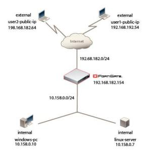
Figure 13: SSL VPN configuration for unique access permissions
