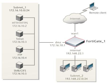
Figure 1: Example SSL VPN configuration
