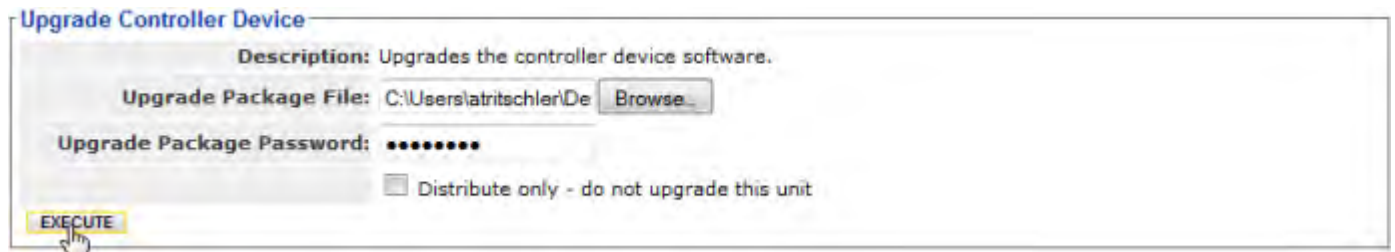
Figure 6.4. Upgrade Controller Device frame, all platforms
