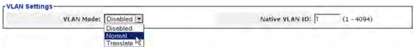
Figure 3.32. Advanced View VLAN Settings frame, all platforms
