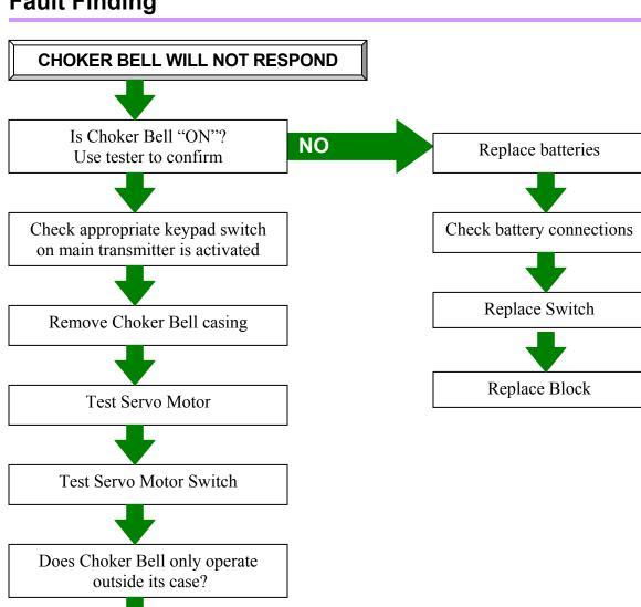
Check aerial connection between aerial button and block. Clean with contact cleaner and add silicon paste.
