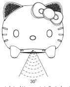
Notes: The remote control should be operated effectively pointing to the nose of KT1, within 6 meters distance and within 60 degrees
