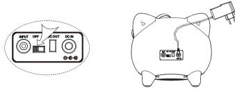
Connect the AC adapter to an AC 120V~60Hz power source. Use the PowerOn/Off Switch to turn the speaker ON or OFF.
