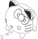
2. Plug one end of the included audio cable into the Aux Input Jack on back of speaker and the other end into the Headphone Jack of your external audio device. Tap the Input button on Hello Kitty's ear to select the AUX Input.
