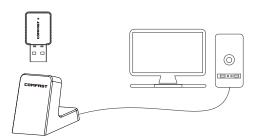
Note: When using the desktop, it is recommended to use the USB extension cable base to connect the rear interface of the computer chassis. (Most of the desktop computer's front USB interface is underpowered or unavailable), extended to the desktopUse, the effect is better!
