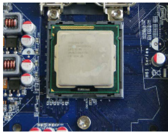
4. Check pin one marking (triangle) with the pin one corner of the CPU socket, align the CPU notches with the socket alignment keys and gently put the CPU onto the socket.
