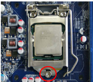
5. When CPU is properly seated, replace the metal cover and push the CPU socket lever back to its locked position.
