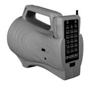
Turn on the Dead Bone transmitter by holding down the power button for about 1-2 seconds. The indicator on the transmitter will illuminate green. When the transmitter begins to get low, the green indicator will flash.
