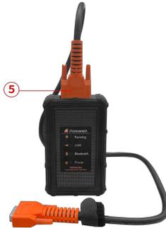
Figure 2-6 Top View of VCI
