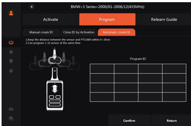
Figure 3-16 Sample Automatic Create ID-The Interface To Detect Sensor
