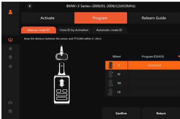
Figure 3-14 Sample Manual Create ID-Programming Completed Interface
