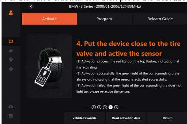
Figure 3-5 Sample Activation Operation Interface
