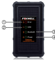
Figure 2-7 Front View of VCI
