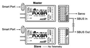
RX8R supports the redundancy function for the master and slave receivers. The master receiver receives SBUS signal from the slave receiver. When the master receiver goes into failsafe, the output signal from the slave receiver will be used until the master receiver works again.
