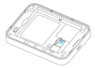
4. Insert the SIM card gently with gold IC chip facing downward
