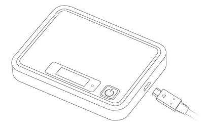
Unplug the AC adapter from the outlet, and remove the micro USB connector from the device.
