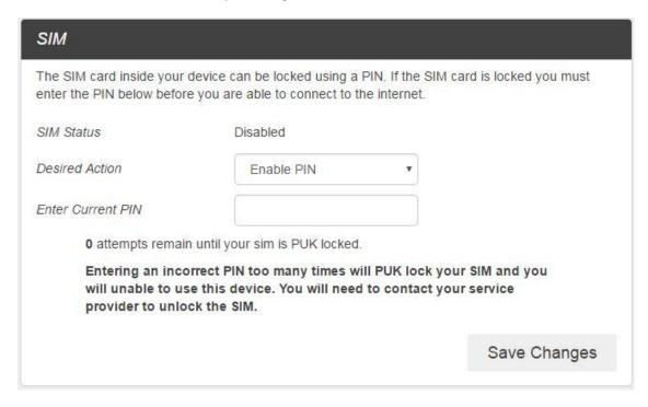
■ Enter the SIM PIN and press "Save Changes". The SIM Status will be changed to Enabled. Once the SIM PIN Lock is enabled, you need to enter SIM PIN to connect to the mobile broadband network each time you power on your R871.
