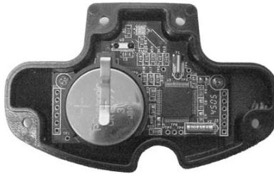
Figure 3. Sirius Wireless Link Opened for Battery Replacement
