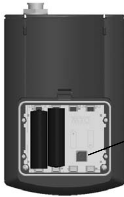
Figure 6. Rotary Switch in Battery Cradle
