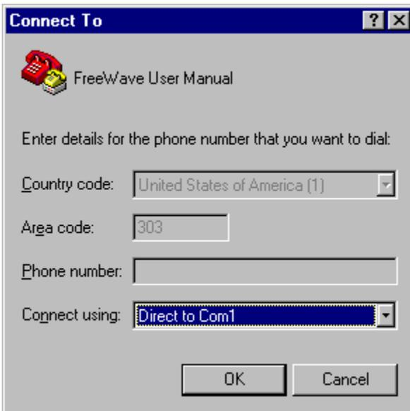
5. Select the connection type to be used from the **Connect using** drop-down menu. In most cases the connection type will be either **Direct to Com1** or **Direct to Com2**.
