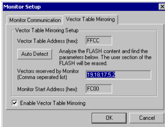
Figure 21.9 Monitor Setup Window - Vector Table Mirroring Tab
