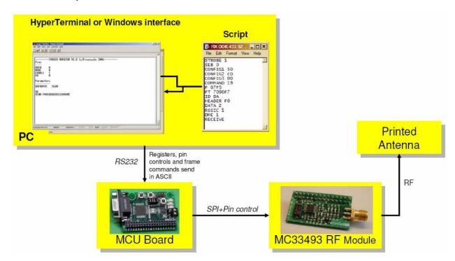
The operation of MC33493 is done by sending with Hyper Terminal a script to the MCU board that will configure MC33493 in a defined configuration.
