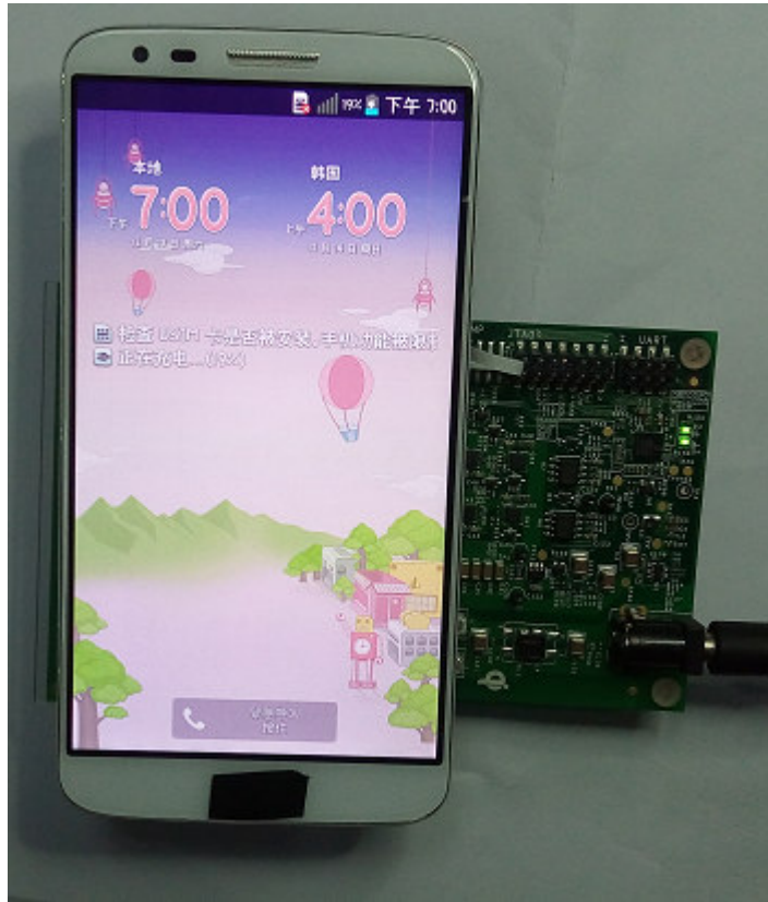
Figure-3 WCT-15W1COILT charging the equipment
