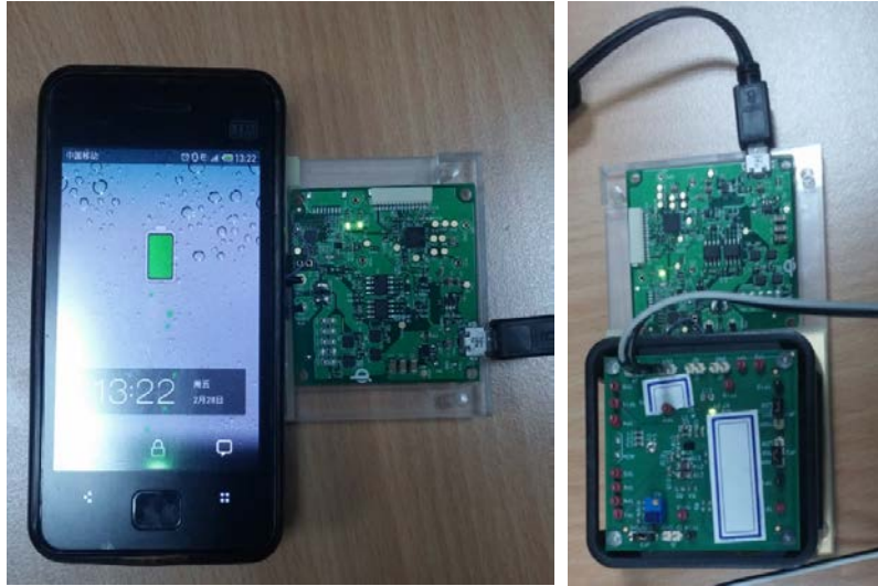
Figure-3 WCT-5W1COILTX charging the equipments
