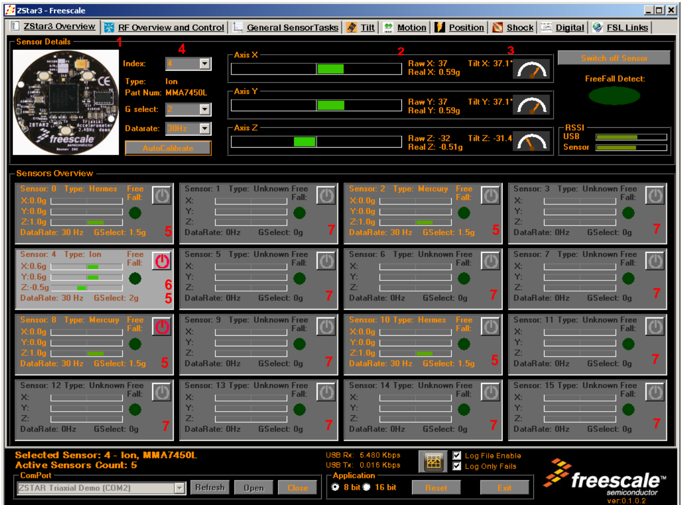
Figure 7-7. Main sensor board overview screen of the GUI
