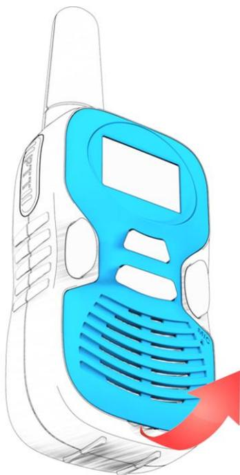
Disassemble the trim from here upwards
