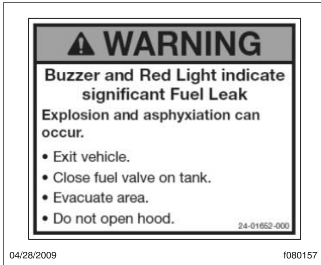
Fig. 25.4, Interior Warning Sticker
