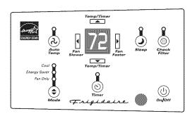
Note: Tap or hold either up(  $\blacktriangle$  ) or down(  $\checkmark$  ) button until the desired temperature is seen on the display. This temperature will be automatically maintained anywhere between 60°F (16°C) and 90°F (32°C). If you want the display to read the actual room temperature. See "To Operate on Fan Only" section on Page 6.
