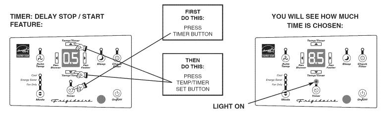
**Note 1:** For Delay Stop, the unit must be in the On position. **Note 2:** For Delay Start, the unit must be in the Off position. First, PRESS TIME BUTTON
