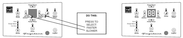
A 2 Digit Display is used to indicate the Fan Speed setting, from 10 through 99. When the "SLOWER" button is pressed the motor speed will slow down at various intervals, down to a minimum setting of 10. To speed the motor up, press the "FASTER" button. The speed will increase at multiple intervals to a maximum setting of 99. Display will revert back to temperature setting after a short time.
