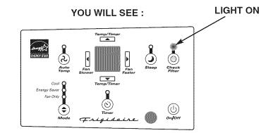
Note: This feature is a reminder to clean the Air Filter (See Care and Cleaning) for more efficient operation and cooling. The LED (light) will illuminate after 250 hours of operation. To reset after cleaning the filter, press the "Check Filter" button and the light will go off.
