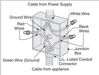
Figure 4 - 4-WIRE GROUNDED JUNCTION BOX
