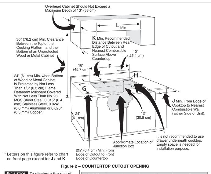
**ACAUTION** To eliminate the risk of burns or fire by reaching over heated surfaces, cabinet storage space located above the cooktop should be avoided. If cabinet storage is provided, risk can be reduced by installing a range hood that projects horizontally a minimum of 5" (12.7 cm) beyond the bottom of the cabinets.
