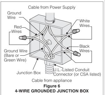
**AWARNING** If connecting to a 4-wire power supply cable electrical system, the appliance frame connected ground wire MUST NOT be connected to the neutral wire of the 4-wire electrical system.
