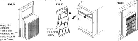
**37 Drill two 9/64" diameter pilot holes** in the top window jamb in line with the partially plugged holes in the panel frame. Secure the panel frame to the window jamb with two #8-32 x 3/4" self-threading screws. If additional holding is necessary, two screws may be used on the sides of the panel frame as well.
