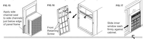
19 Slide inner window sash firmly against side of the cabinet. Make sure not to peel the seal strips from the window track and cabinet side channels. If the panel frame does not fit snugly to the inner window sash, secure the panel frame to the sash with #8 x 3/4" self-threading screws. Use the partially plugged holes in the panel frame. Drill 1/8" pilot holes for the screws.
