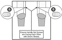
Matching Refrigerator and Freezer Door Handle Installation
