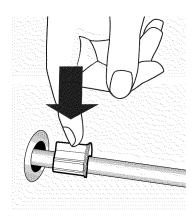
3. Slide the shelf grommet into the grommet already in the freezer wall until it is flush.
