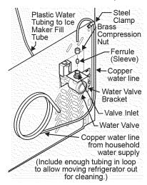
Plastic Water Tubing to Ice Maker Steel Clamp
