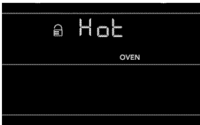
Figure 34: Hot oven after clean with door still locked
