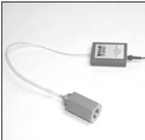
Figure 6.3.5A Insert earphone attached to coupler
