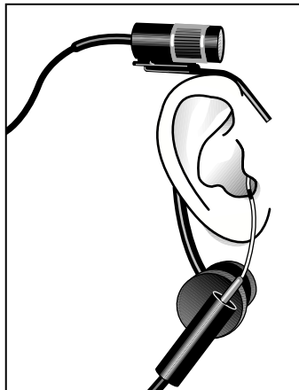
Figure 6.2.2—Placing the reference and probe microphones
