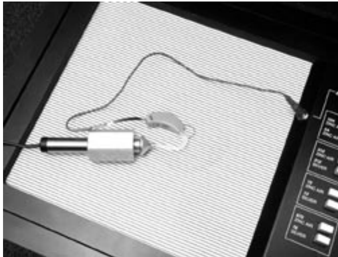
Figure 3.3.3—Behind-the-Ear Aid with Ear-level Adapter
