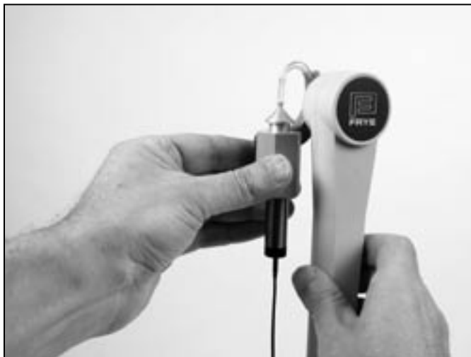
Figure 5.1.4—Holding telewand parallel to the body of a BTE
