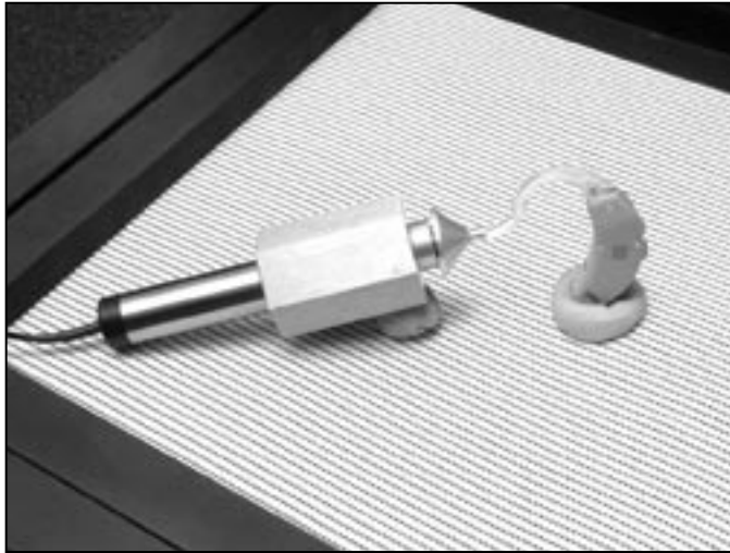
Figure 3.4.10A—Testing with the Sound Chamber Telecoil Board
