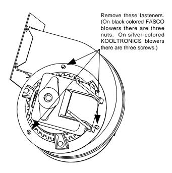
3. Wrap the motor with plastic wrap to prevent water from entering it. Spray degreaser or detergent on the blower wheel and the blower housing. Allow it to soak for five minutes. Rinse the wheel and housing with hot tap water, then dry with a clean cloth.
