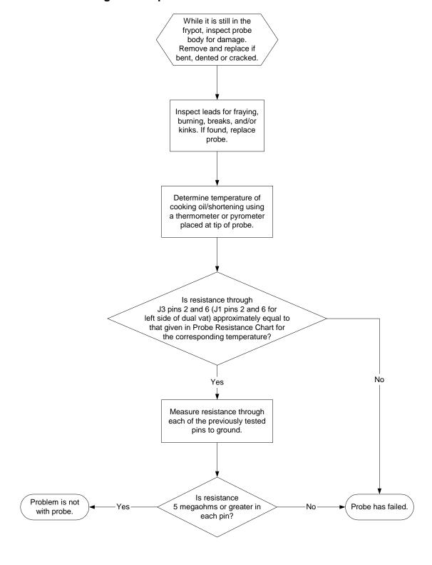
**Note**: Disconnect computer before measuring probe resistance.
