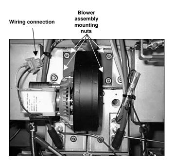
2. Remove the three fasteners that secure the blower motor assembly to the blower housing, and separate the two components.
