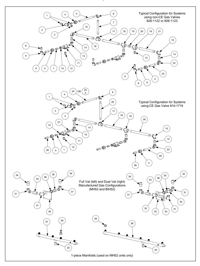
**NOTE:** The drawings on the preceding page illustrate typical gas manifold configurations. Specific configurations vary depending upon the number and types of fryers in a battery. The purpose of the drawings is to illustrate all individual components that may be found in any given configuration. Determination of which component to use in a particular application should be based upon careful inspection of the existing components, including taking measurements when appropriate.
