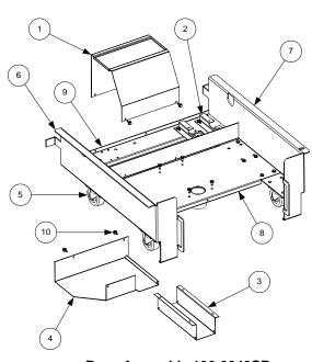
Base Assembly 106-0043SP (Replaces Base Assembly 806-5985 used on units built prior to August 1997)
