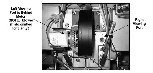
The air/gas mixture is properly adjusted when the burner manifold pressure is in accordance with the applicable table on page 3-7 and the burners display a bright orange-red glow. If a blue flame is observed, or if there are dark spots on a burner face, the air/gas mixture requires adjustment.
