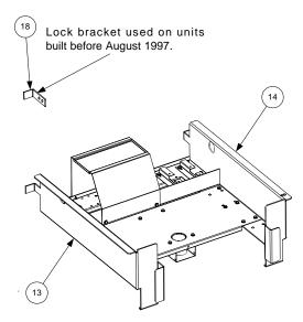
Base Assembly 806-8648SP (Used on units built August 1997 and later.)
