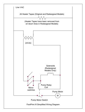
For FootPrint III systems built before August 1997, all heater tapes are wired directly into the line VAC source. They remain energized as long as the unit is plugged in. In systems built in August 1997 and later, oil return line heater tapes have been eliminated. In these units, the only heater tape used is on the suction tube and pump. This tape is still wired directly into the line voltage. A pair of vacuum-breaking solenoids is wired into the 24VAC circuit.
